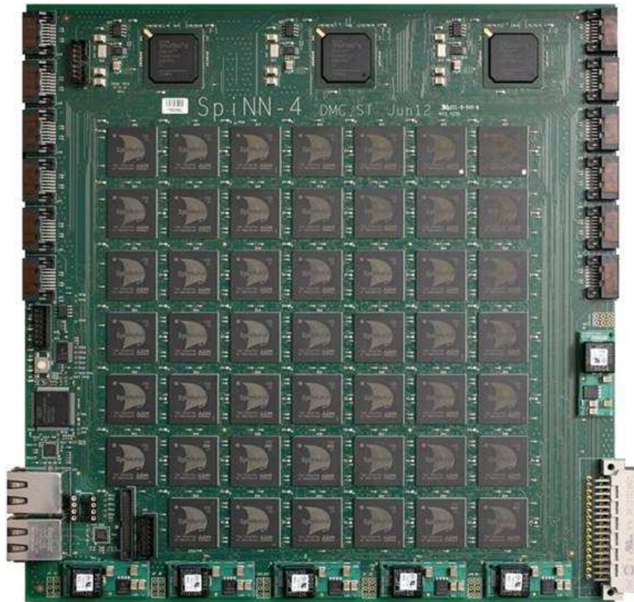
Figure 2.2: The 48-node SpiNNaker board
