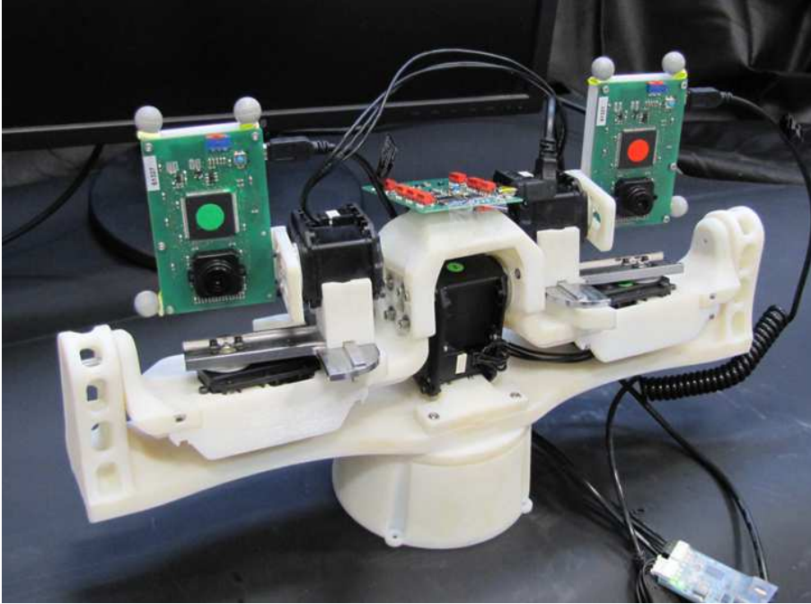
Figure 2.1: The Robot Head with the two eDVS sensors.
